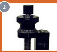
To aid speed in changing the height adjustment I like to cup the knob in the palm of my open hand and turn it this way. With some practice this is much faster than gripping in with your fingers. The new large dial gets in the way of this a little due to its greater diameter. I plan to add a spacer below the knob so it sits a little higher off the dial and I believe that this will remedy this slight inconvenience.
