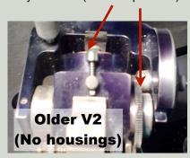
keep polishing powders, gemstone grit, and other debris from falling into some of the vital parts of the machine and increases machine life. It is a very positive change, especially for those who cut a lot.
